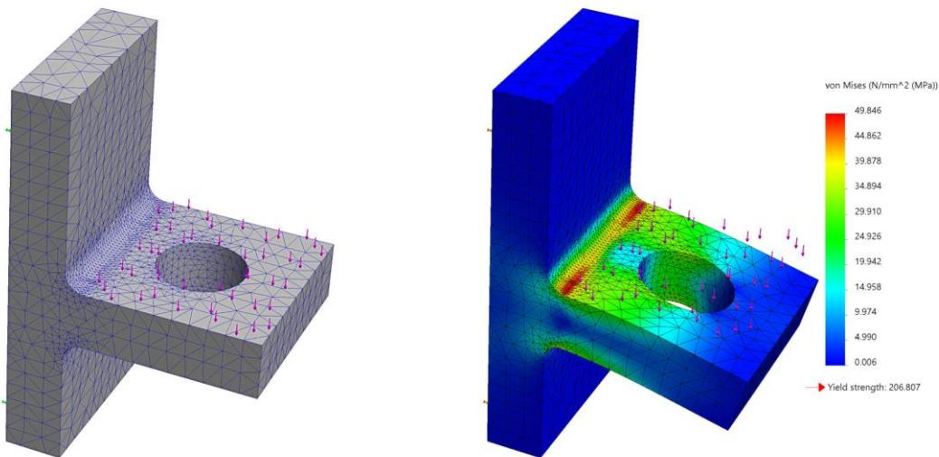
In the photo above, the red parts show where this part is most stressed and the blue parts show where the part is the least stressed. As the connection point is where the most stress occurs, you can see it bends a little downwards.
